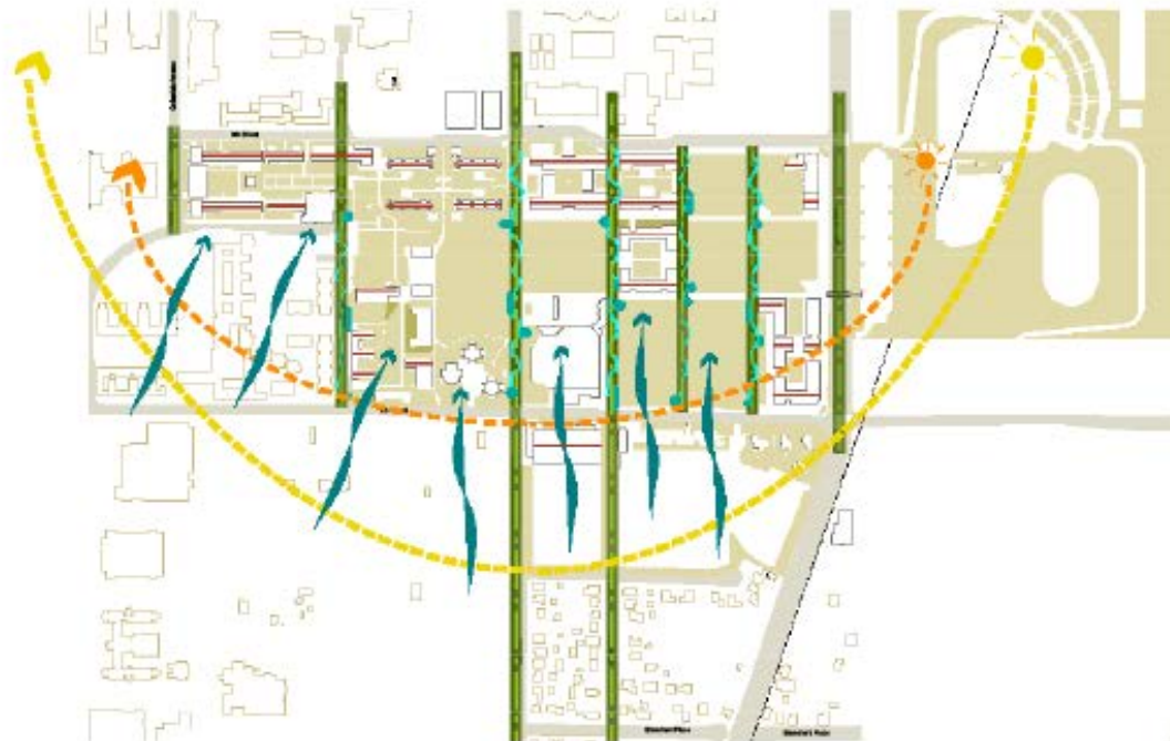
Site Analysis: Sun path, prevailing winds, optimum orientation and green corridors
